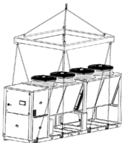
Fig. 7 Unit handling by crane
